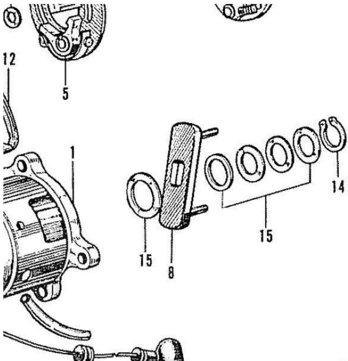
**EN:** To install the 123/TUNE+ Honda S800, you must transfer the drive dog <sup>(8)</sup> from the original distributor, together with the spacer rings <sup>(15)</sup> and circlip <sup>(14)</sup>. Make sure that the drive dog does not touch the ignition housing when mounted (spacer rings are important)!
